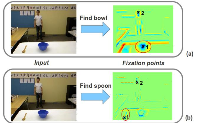
Fig. 2. Output of the algorithm: (Left) Input scene. (Right) Top two fixation points (black crosses with corresponding ranks) for the two target objects: (a) bowl and (b) spoon, computed using known properties of the target objects.
