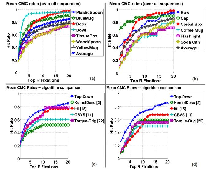
Fig. 8. [Top row] (a) & (b): CMC curves for all objects of the proposed algorithm ‘Top-Down’ averaged over all sequences. [Bottom row] (c) & (d): Comparing averaged CMC curves over all objects from both datasets from all algorithms. Left column: `UMD-clutter`, Right column: `rgbd-scenes`.
