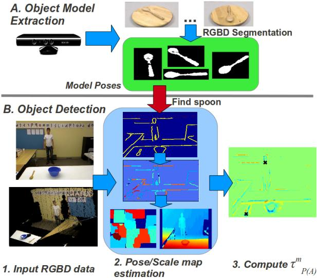
Fig. 6. Overview of the proposed top-down object detection algorithm. (A) Extracting object model properties from RGBD data: poses and size. (B) Runtime detection of target object: (1) Input RGBD data. (2) Compute pose and scale maps using object model information. (3) Compute  $\tau_P^m$  and find extrema (the top 2 absolute extrema values are shown as black crosses).
